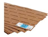
Natural cork mat for improving footfall sound insulation with cut-outs for accommodating WAKOL MS 232 Parquet Adhesive, elastic or WAKOL MS 262 Parquet Adhesive, firm-elastic, and suitable for laying strip parquet and solid wood planks up to max. 18 cm in width and multi-layer parquet as of 90 cm in length as well as for cork on HDF/MDF carrier with tongue and groove joining or click joining on absorbent and non-absorbent subfloors indoors.
