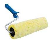
Polyamide roller for applying WAKOL MS 330 Silane Primer when used as moisture barrier, for priming on strong absorbent subfloors, old subfloors and adhesive residues. Also suitable for applying WAKOL PS 275 Concrete Repair
