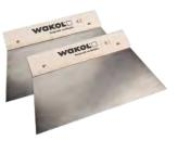
Notched trowel according to TKB for applying Wakol dispersion adhesives. WAKOL Notched Trowels are available in notch sizes TKB A1 and TKB A2 with 25 cm width and in notch sizes TKB B1 and TKB B2 with 18 cm width.
