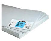
Polyester fibre sheet for decoupling and soundproofing reduction under bonded parquet indoors also appropriate for applying a levelling layer before bonding textile and elastic flooring.
